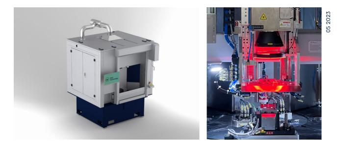
More and more power tools and gardening equipment are being built with compact and lightweight battery systems thanks to new battery technologies. Without cables to the power socket, they can thus be used on the move and enable efficient, ergonomic work. In manufacturing, laser welding is used in the assembly of battery modules, especially for cell contacting. The contacting of battery cells by laser is characterized by high reliability and low costs per cell.
