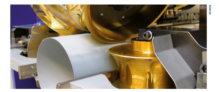
Production centre for medium short tubes with integrated multi roller roll-former
